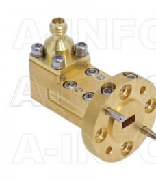
15WCA1.0_Cu Right Angle Rectangular Waveguide to Coaxial Adapter 50-75GHz WR15 to 1.0mm Female
